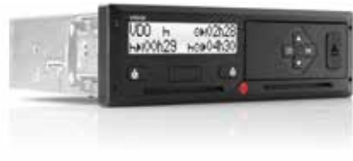
■ Abb. 2.1 VDO-Kontrollgerät DTCO 1381, Release 2.2 (© Continental)
